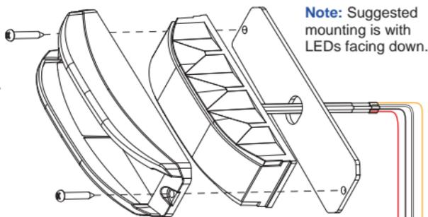
**Note:** Suggested mounting is with LEDs facing down.
