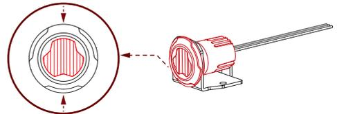
**NOTE:** Optical stripes must align vertically to meet regulation.
